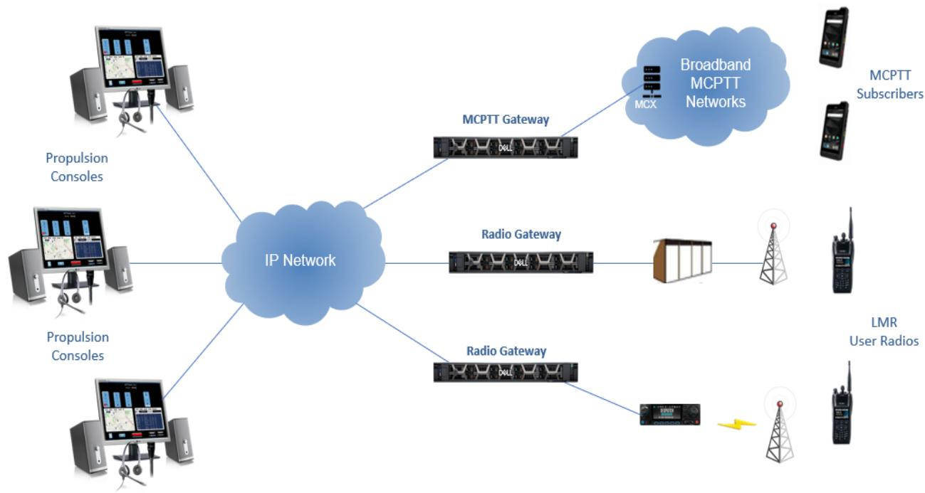
**Propulsion™** communicates over Internet Protocol (IP) based networks with radio Gateways that transmit and receive voice and control radio systems. These radio Gateways control the widest variety of radio resources in the industry:
