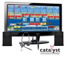
Propulsion is a graphics rich, critical voice dispatch console for Digital Mobile Radios (DMR), that also provides interoperability with Project 25 radios, MDC, and other radio formats. This scalable product provides integrated instant call recording and optional telephone interconnect (SIP or POTS).
